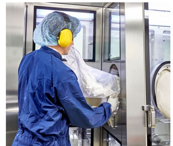
Component transfer at customer site (courtesy Octapharma) DPTE-BetaBag® was first sterilized in a Getinge sterilizer.
