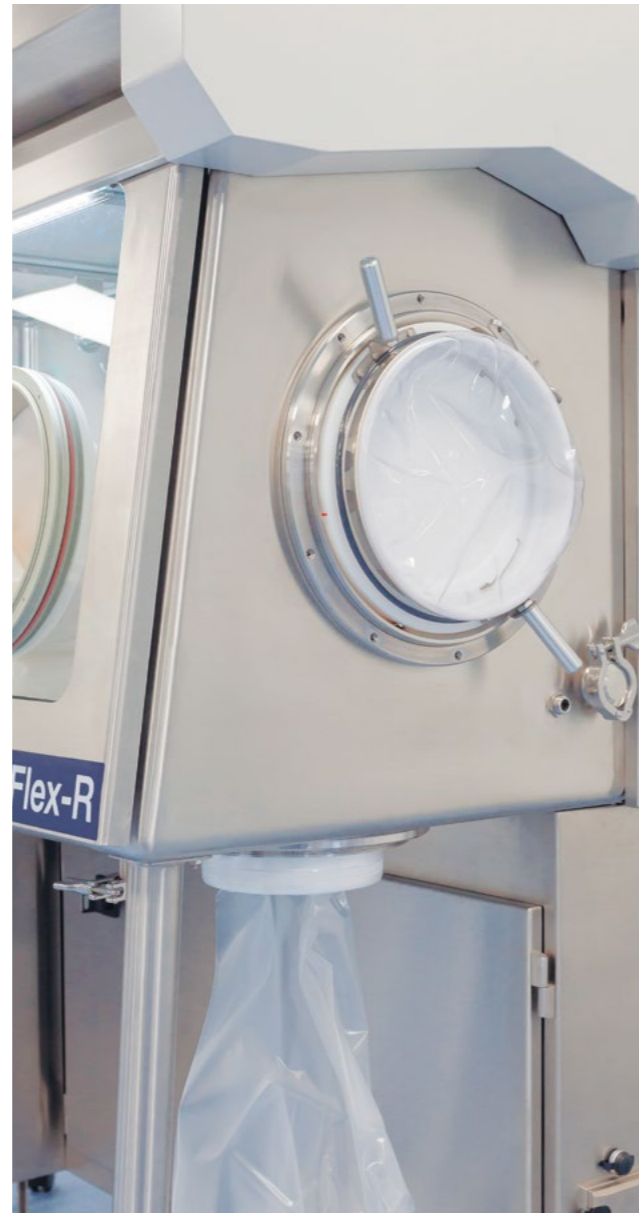
Waste removal from an isolator using a DPTE-BetaBag®
