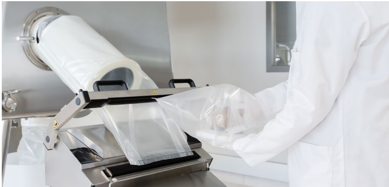
DPTE® Tubing with heat sealing machine for removal of items from the sterile zone
